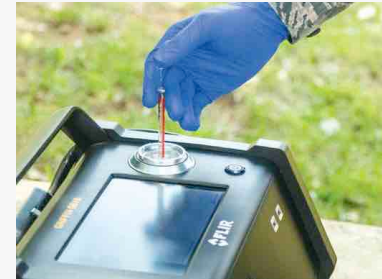
Portable GC/MS in the field.
